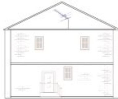
Most antennas can be installed in attics or overhead crawl spaces, if there isn't too much foil insulation or metal roofing material present.
