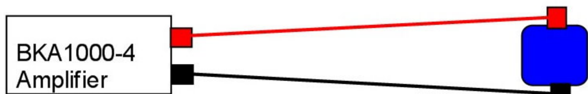
1 BK-LFE wired to BKA1000-4 = 4 Ohm Load
